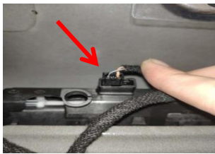
3.14 接中控开关控制线：尾门原车开关按钮内侧插头；注意箭头和拍摄视角
